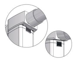
Step 1 - Pull the lock bar down to release from stop position.
