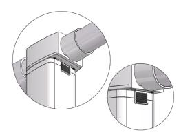
Step 3 - Release the lock bar and make sure it is in the stop position.
