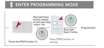
Please select channel for multi-channel remote before operation as 0.5 seconds is needed for up/down converting, max single running time is 4min.
