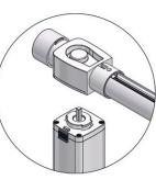
Step 1 - Pull the lock bar down to release from stop position and twist to remove motor.
