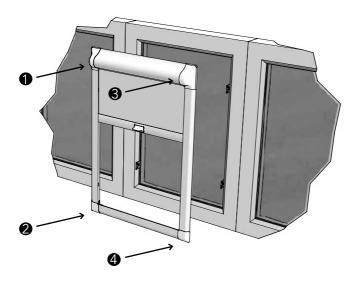
Firmly press the frame down onto each bracket. Fit one side at a time for an easier installation, 1, 2, 3, 4.
