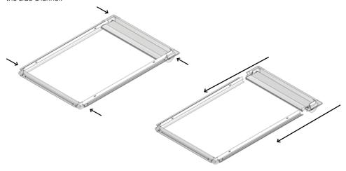
To ensure all brackets are in the correct position for fitting (85mm from beading) use a credit card in the corner of the window to locate the bracket position.
