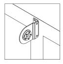
Place an intermediate bracket at the intermediate point 2mm less than the size taken, ensuring the central face of the intermediate bracket lines up accordingly.
