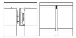
11. Adjust the blind to be level with the control blind. Depress the coupling plunger until the blind is free to turn, (drive connector and coupling fixed end disengage) turn blind until bottom bars are level.
