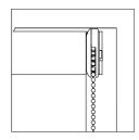
6. Locate, insert and secure control end.
