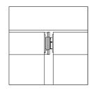
8. Depress the coupling plunger and then locate and secure fixed end into first blind.
