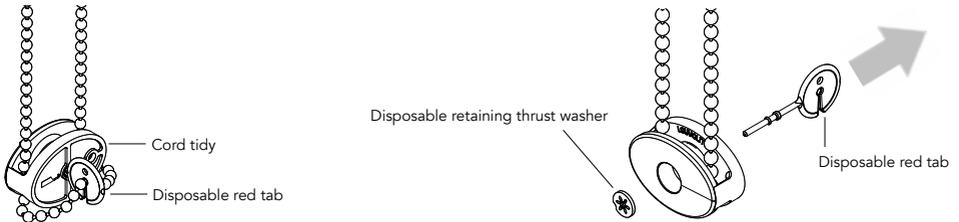
Position the cord tidy to the wall at the furthest distance below the roller tube adding appropriate tension to the chain and mark its location.
