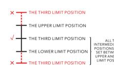
ALL THE INTERMEDIATE LIMIT POSITIONS MUST BE SET BETWEEN THE
