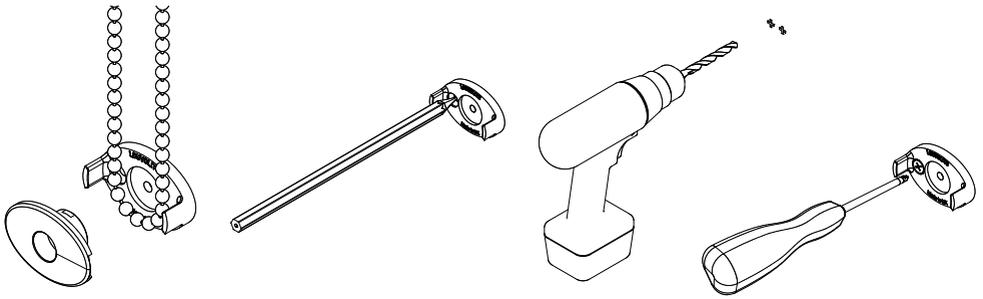
Re-assemble the cord tidy with the chain and fix it in previously marked position with a screw through the centre hole.
