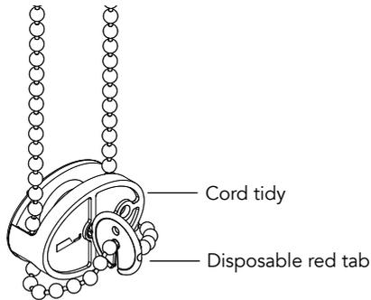
Remove the disposable red tab by disengaging it from the chain and then pull out the disposable red tab.
