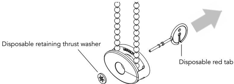
Position the cord tidy to the wall at the furthest distance below the roller tube adding appropriate tension to the chain and mark its location.
